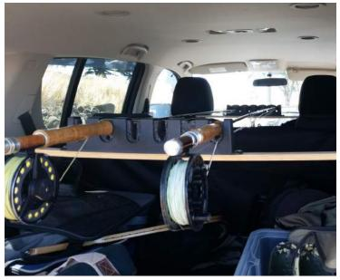
Constructed using rod holder from tackle shop (\$15 approx.), timber, threaded nut and bolts, and two tile holders. I drilled a slotted hole to allow the suction cup to move along the wood and then to be tightened after adhering to the rear window.
