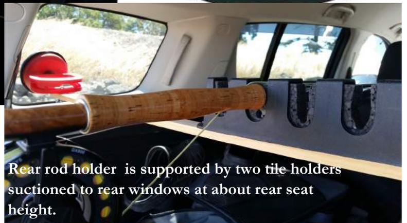
Rear rod holder is supported by two tile holders suctioned to rear windows at about rear seat height.
