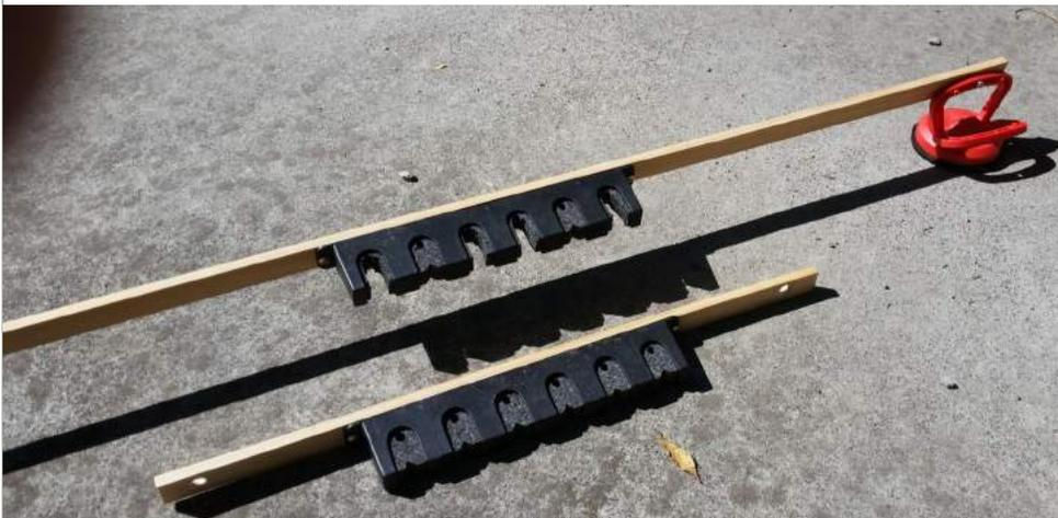
Constructed using rod holder from tackle shop (\$15 approx.), timber, threaded nut and bolts, and two tile holders. I drilled a slotted hole to allow the suction cup to move along the wood and then to be tightened after adhering to the rear window.
