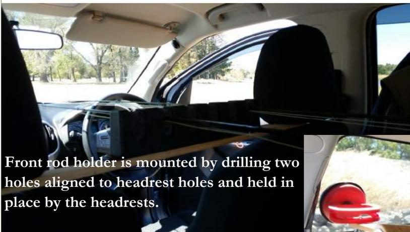
Front rod holder is mounted by drilling two holes aligned to headrest holes and held in place by the headrests.
